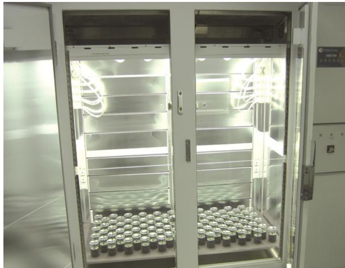
FIGURE 1. Experimental setup of a single experiment in the growth chamber (100 beakers with L. gibba ). For every experimental parameter ( n = 20 in total), five replicates were used and allocated in a fixed-blocked randomization scheme. The 20 experimental conditions consisted of 18 letter-coded samples and two additional open controls, one with unimpaired duckweed and one with duckweed impaired during the entire experimental interval (the latter two controls were not used for the statistical evaluation).
